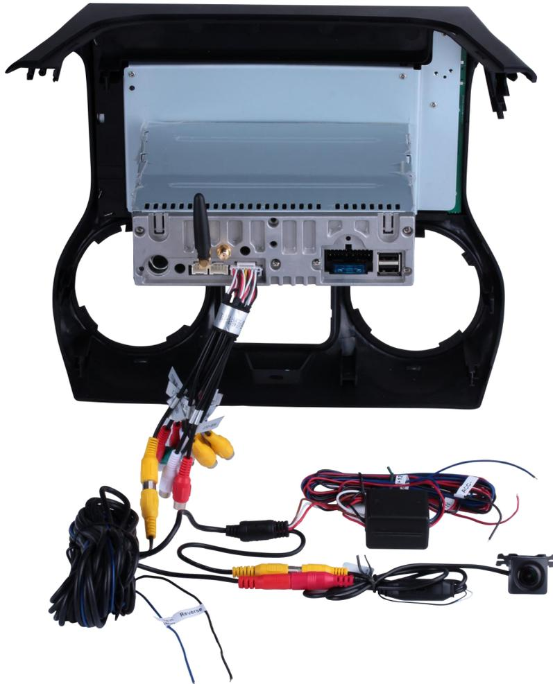
Here shows you the wiring of wireless rear view camera.
