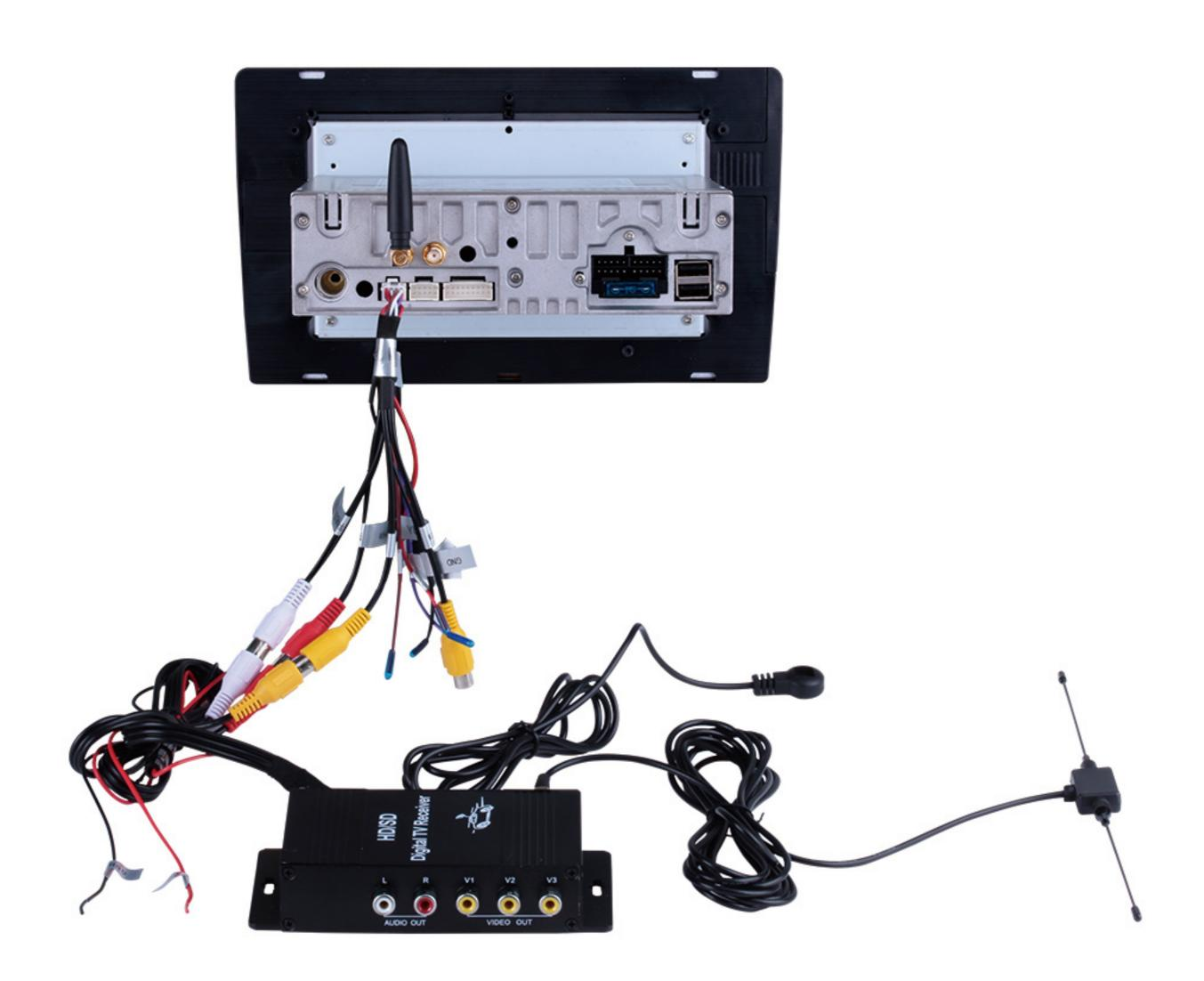
You can click into TV after the installation of ATSC, DVB-T and ISDB. Here is an Screen-shooting after ATSC installation.
