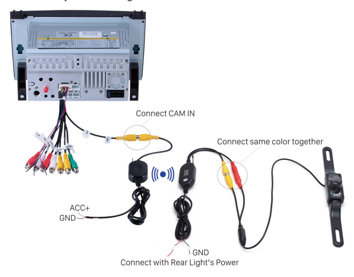
If you still can't get reversing camera image at reverse gear after installing your wireless camera according to the above way, please find and connect the brown "CCD AV IN" cable (or REVERSE cable in the supplied power harness) to + positive of your reverse lamp.
