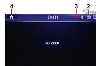
1. Touch to turn off the screen. When the screen turned off, touch any portion of the screen to turn on the screen.
