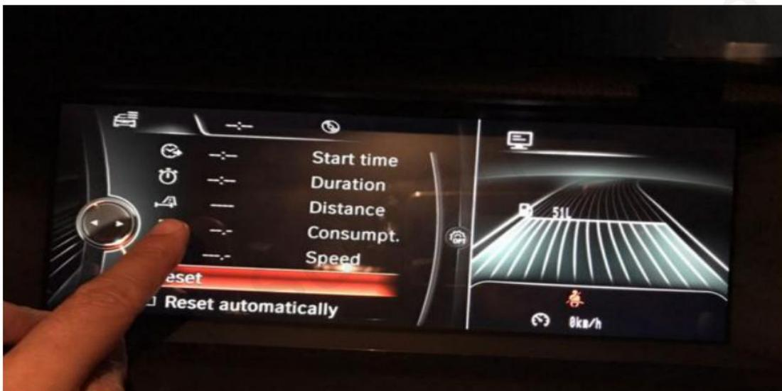
Reason: Did not remove the optic fiber from Original power harness and plug it into our power harness.
