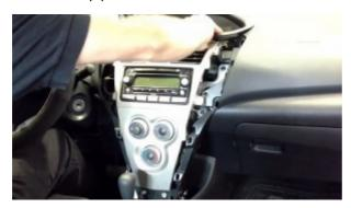
3. Remove 4 screws holding the unit with a Phillips screwdriver.
