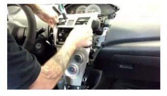
5. Take out the radio and disconnect cables at back of it.
