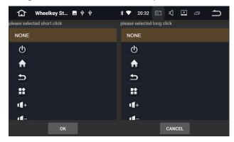
Enter the setting interface to select key learning, "steering wheel control reset" firstly,then long press the buttons on the steering wheel,select the corresponding keys in the interface, When the setting is successful, the corresponding buttons of interface will light up.
