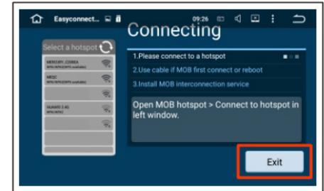
2 Wifi connection, turn on the "Easy connection Application", select wifi connection icon, then creat a wifi hotspot on headunit, after that connect mobile to the hotspot. then screen mirror will appear.
