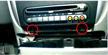
3.Gently pry around the side of trim panel with the lever and then remove the trim panel.
